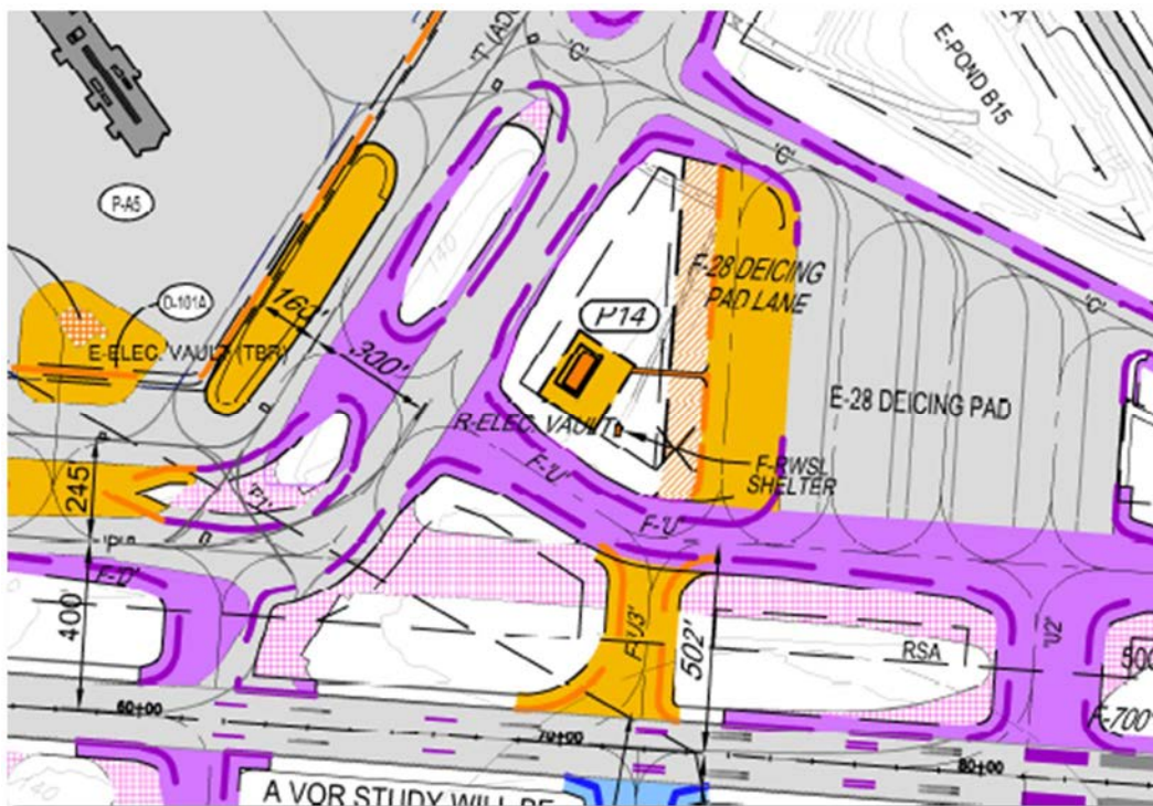
Figure 26: Relocate Airfield Lighting Vault
